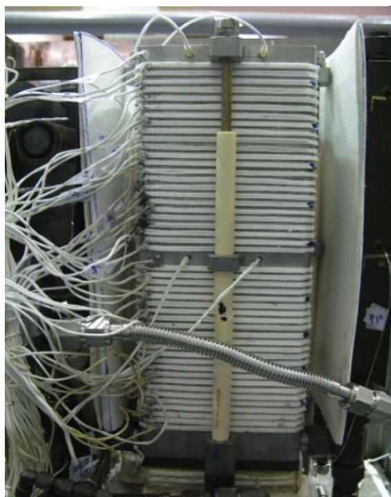
Fig. 3 – Photograph of a 1 kW SOFC stack.
