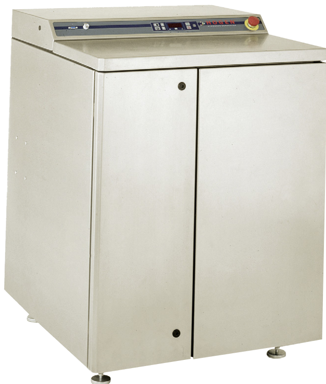
FIGURE 2.14 PEM electrolyzer HOGEN S Series by Proton OnSite. Productivity, 1 \text{ m}^3 \text{H}_2/\text{h} ; electric power consumption, 5.6\text{--}9.0 \text{ kWh}/\text{m}^3 ; electrolysis voltage, 2.3\text{--}3.8 \text{ V} ; output pressure, 1.4 \text{ MPa} ; size, 97 \times 78 \times 10^6 \text{ cm}^3 ; weight, 215 \text{ kg} . (For color version of this figure, the reader is referred to the online version of this book.)
