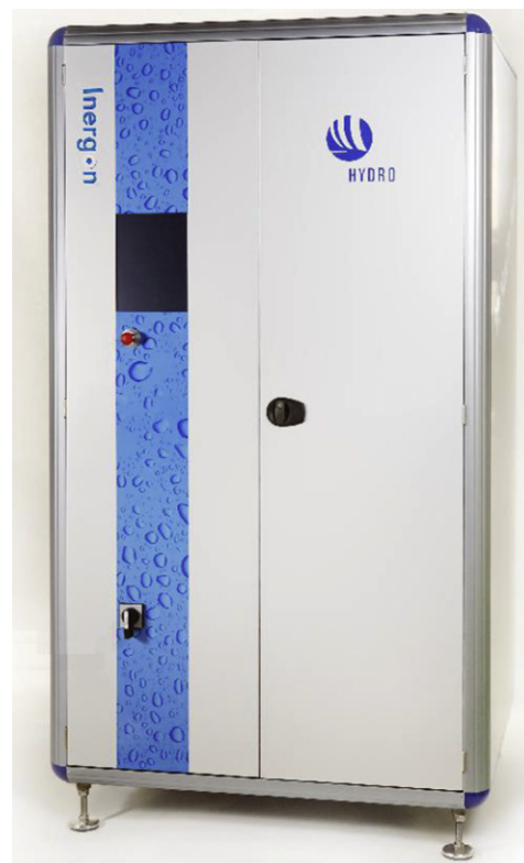
FIGURE 2.15 PEM electrolyzer by Yara (Norsk Hydro Electrolysers). Productivity, 10 \text{ Nm}^3 \text{H}_2/\text{h} ; electric power consumption, 4.4 \text{ kWh}/\text{m}^3 ; output pressure, 3.0 \text{ MPa} ; hydrogen purity, 99.9\% ( \text{O}_2 as main impurity). (For color version of this figure, the reader is referred to the online version of this book.)
