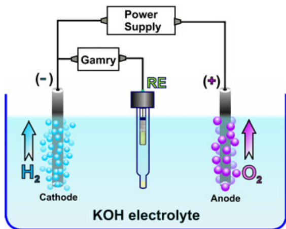
FIGURE 1 Illustration of the desktop water electrolysis experimental setup. RE, reference electrode [Colour figure can be viewed at wileyonlinelibrary.com ]
